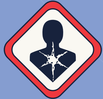
Serious health hazard
